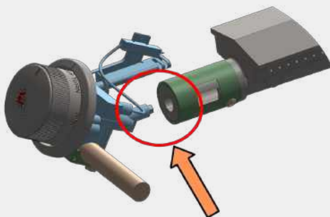
INCORRECT POSITION (NOTE GAP BETWEEN BURNER TUBE AND BURNER ORIFICE)
